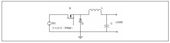
Figure 1-2 Simplified Buck Circuit
